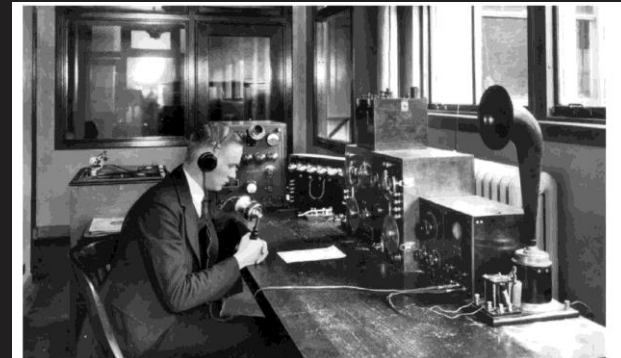
This is what the Detroit News station WWJ in Detroit, Michigan, looked like in 1920. The de Forest 50-watt transmitter is in the center of the image, to the left of the operator, Fred Luthrup. (Detroit News collection)
