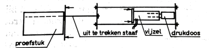
Figure 4.2: Test setup of the experimental research performed by CUR 23
