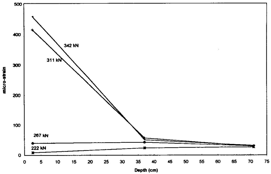
Figure 14 Transverse Bar Strains for an Offset Spacing of 15 cm (6 in.).
