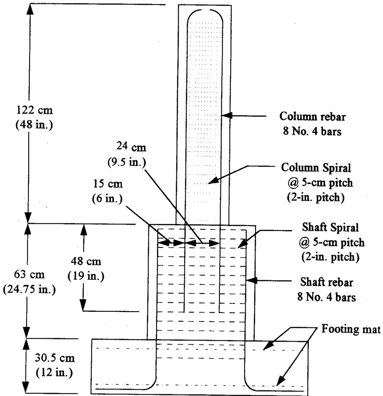
Figure 6 Column-Shaft Flexural Specimen Details.
