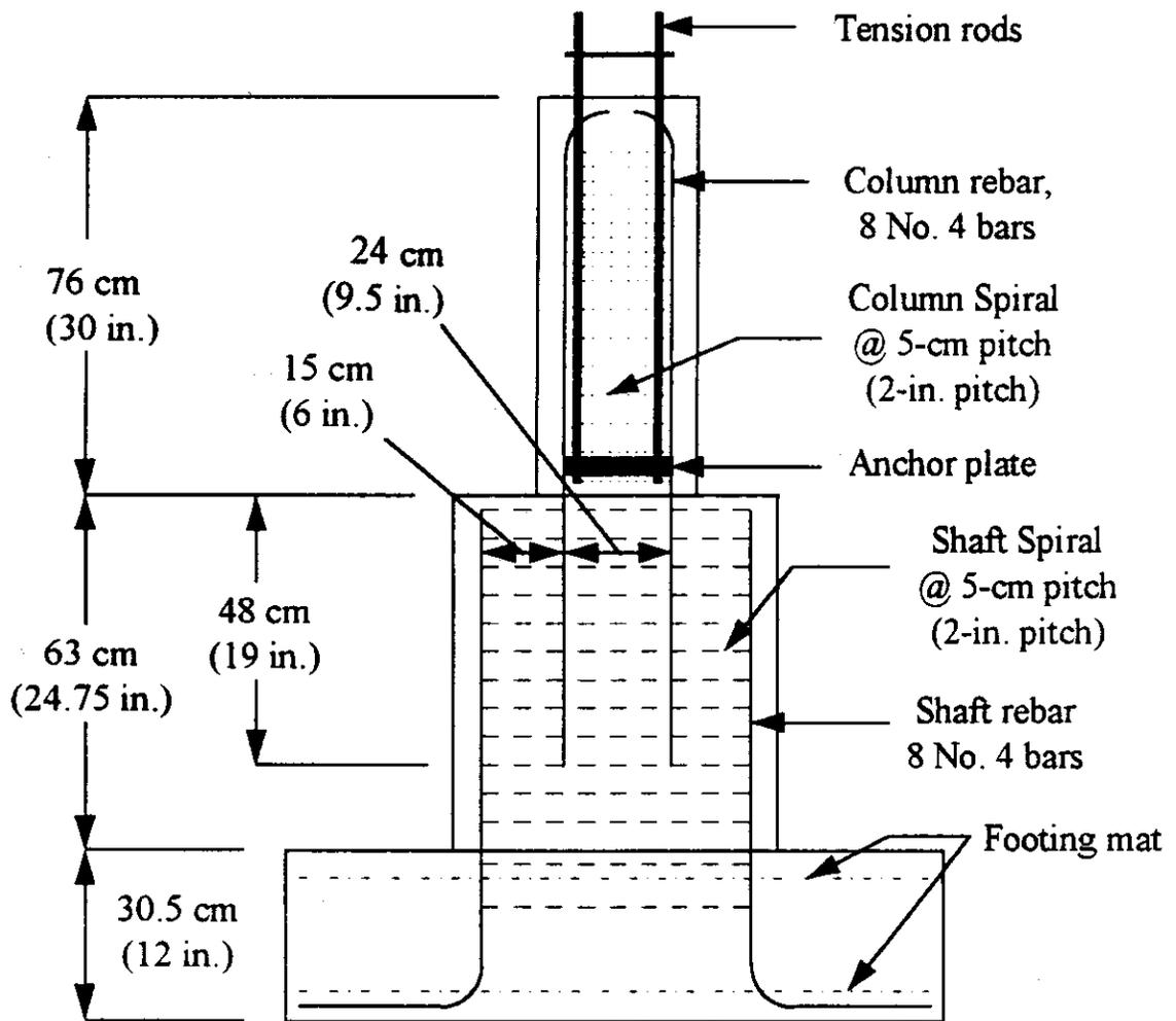
Figure 5 Column-Shaft Tension Specimen Details.
