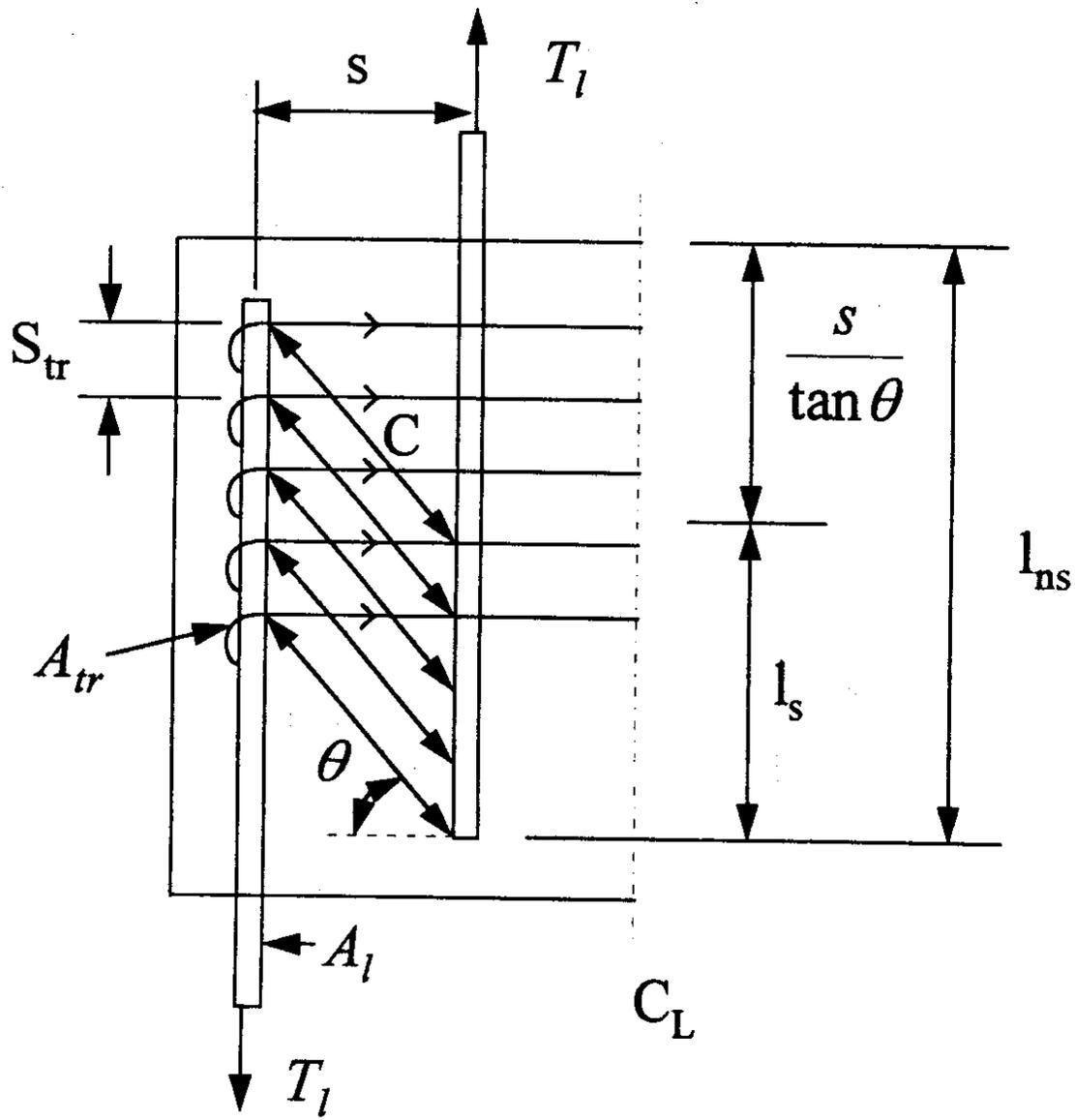
Figure 2 Proposed Two-Dimensional Behavioral Model for Noncontact Lap Splices.
