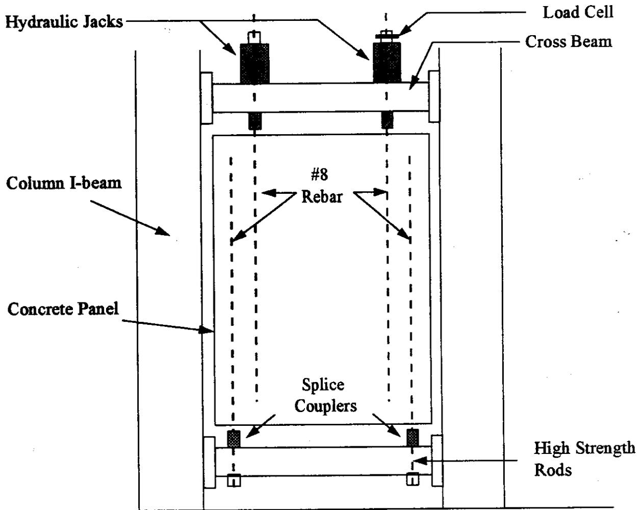
Figure 7 Panel Testing Setup.
