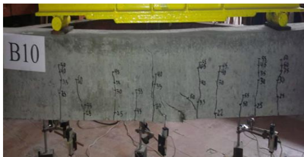
Figure 2.3: Experimental setup by Abdel-Kareem et al (2013) comparable to Ragi Aly (2007).
