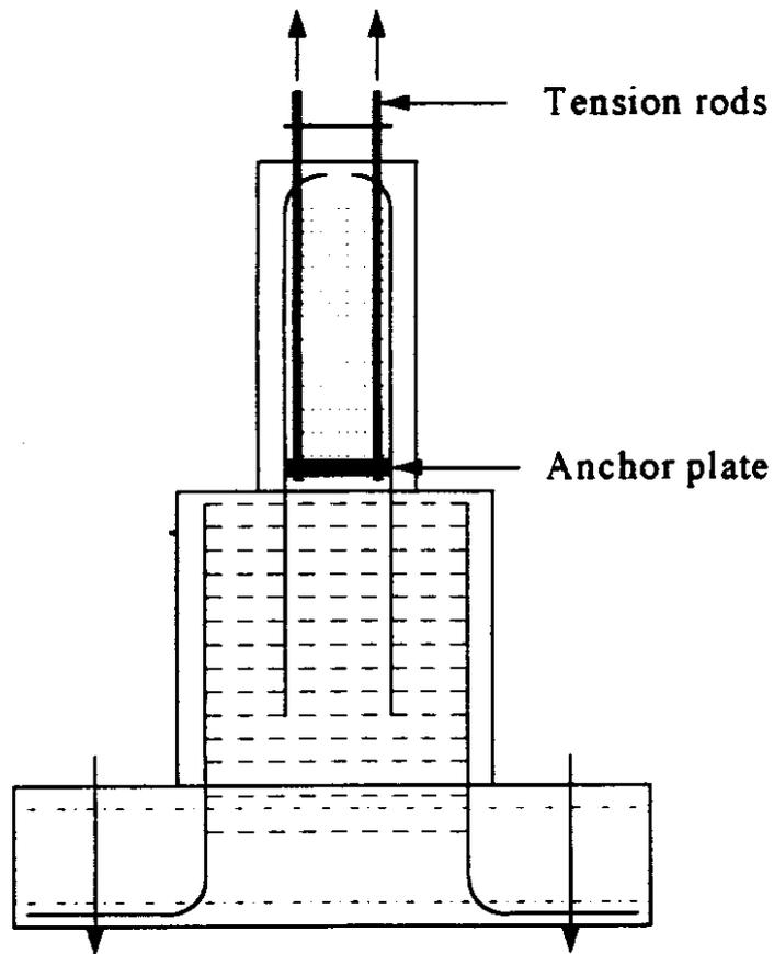
Figure 8 Column-Shaft Tension Testing Setup.
