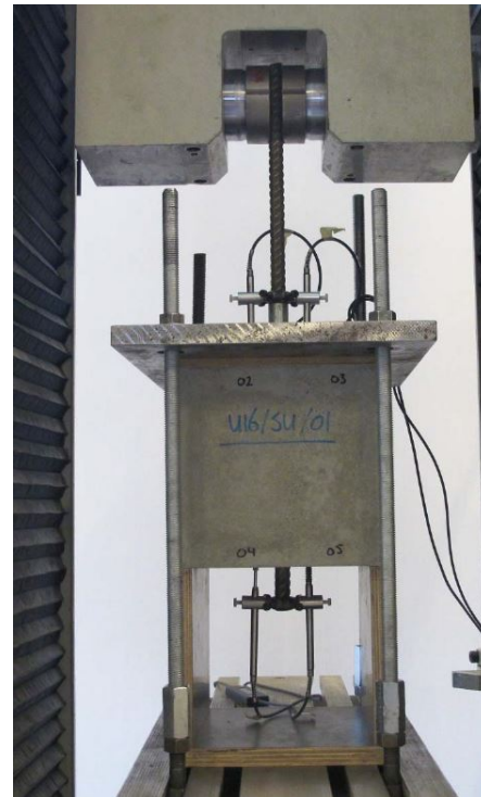
Figure 12: Setup according to RILEM RC-6
