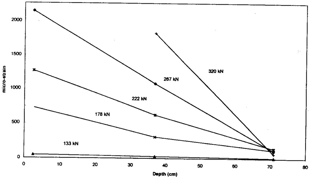
Figure 15 Transverse Bar Strains for an Offset Spacing of 38 cm (15 in.).
