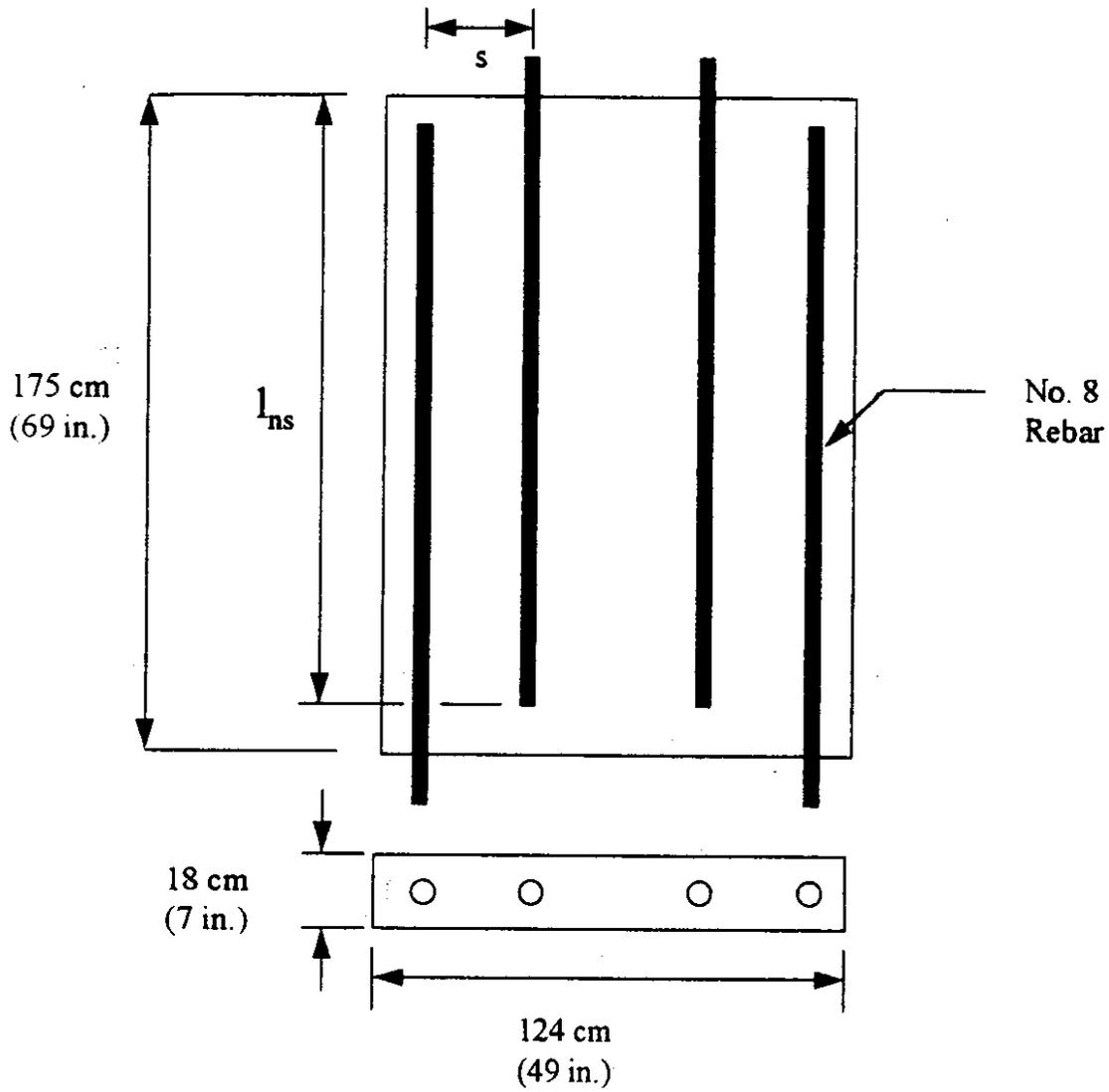
Figure 4 Panel Specimen Details.
