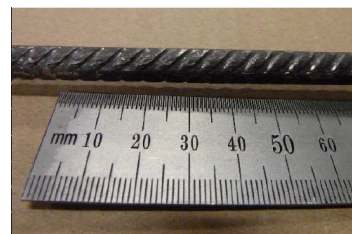
Figure 9: Geometry of Ø8 mm
