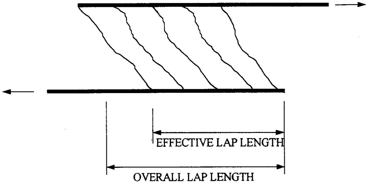
Figure 1 Effective Lap Length (Adapted from Sagan, et al, 1988).
