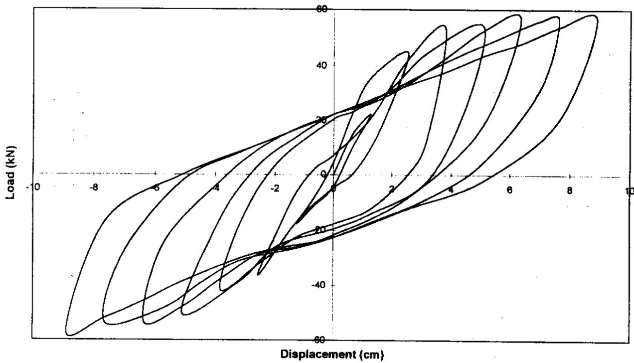
Figure 17 Load vs. Displacement Hysteresis Curves for the Column-Shaft Flexural Specimen.
