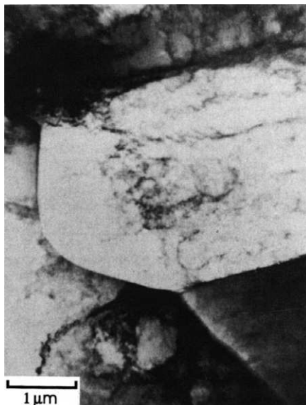
Fig. 7.28. TEM micrograph of SIBM in copper deformed 14% in tension and annealed 5 min at 234°C, (Bailey and Hirsch 1962).
