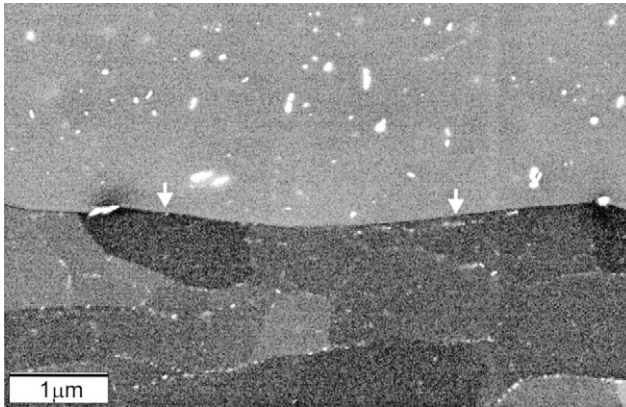
Fig. 9.25. Preferential coarsening of incoherent \text{Al}_3\text{Zr} particles at a HAGB migrating in the marked direction during recrystallization on slow heating to 350^\circ\text{C} , (Humphreys et al. 2003).
