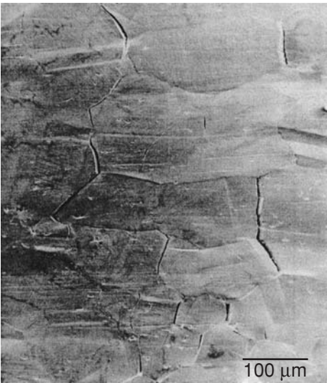
Figure 16.10. Grain boundary cracking in UPH Ni-16Cr-9Fe after 35% elongation at 350°C. From R. W. Herzberg, Deformation and Fracture Mechanics of Engineering Materials , 4th ed., Wiley (1996).
