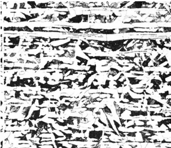
Figure 13.12. Microstructure of a steel plate consisting of bands of pearlite (dark regions) and ferrite (light regions). From Metals Handbook , v. 7, 8th ed., ASM (1972).
