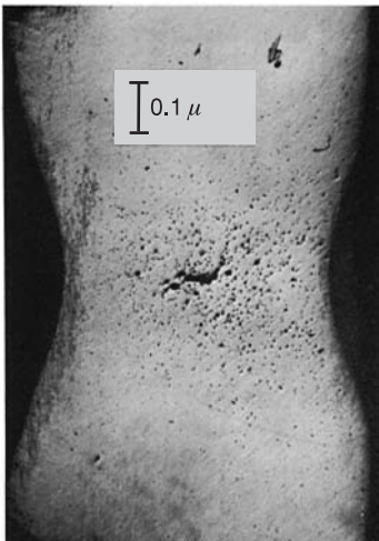
Figure 13.4. Section through a necked tensile specimen of copper, showing an internal crack formed by linking voids. From K. E. Puttick, Phil Mag. , v. 4 (1959).
