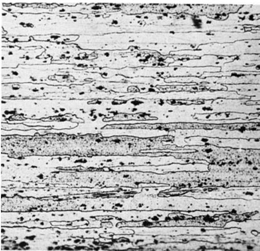
Figure 13.11. Directional features in the microstructure of 2024-T6 aluminum sheet include grain boundaries, aligned inclusions, and elongated inclusions. From Metals Handbook , v. 7, 8th ed., ASM (1972).
