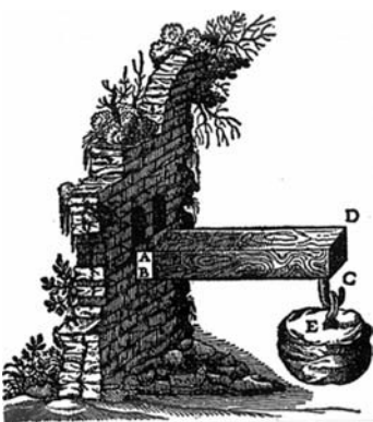
Figure 3.34. Galileo’s sketch of a bending test.
