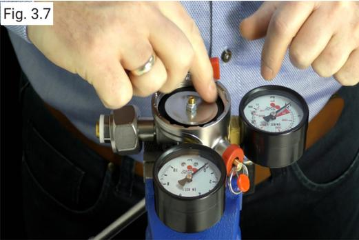
Be sure to push the new Diaphragm to the bottom of the regulator housing.
