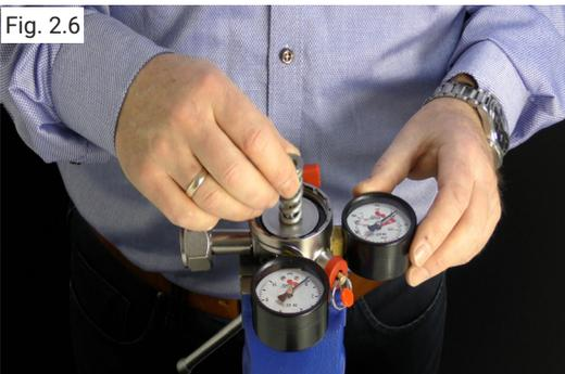
Remove the spring disc and the setting spring.
