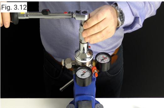
Place the service tool and tighten it with a torque of 33 Nm ( $\pm 3$  Nm) by using a torque wrench.
