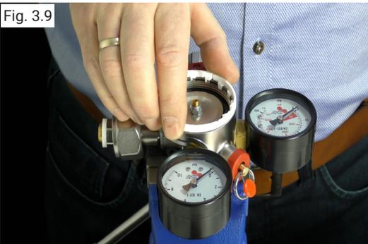
Fit the new Tamper evident ring - orientated as shown on the picture.
