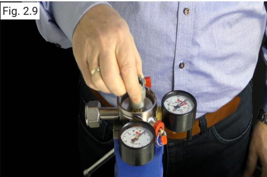
Place the service tool, so that it locks into the geometry of the Cartridge.
