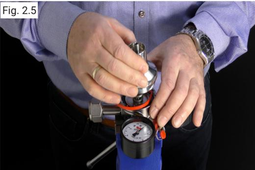
Release the Bonnet completely by hand – the Bonnet is to be reused.
