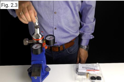
Place the service tool, so that the four grooves fits the four ribs on top of the Bonnet.
