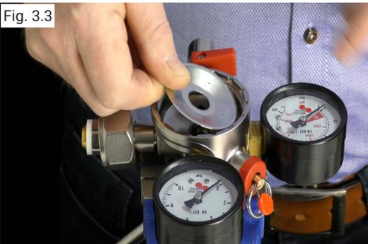
Place the reused Baffle plate as shown on the picture.
