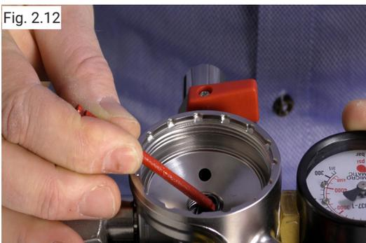
Remove the old o-ring by using the o-ring installation tool from the kit. Scrap the o-ring.
