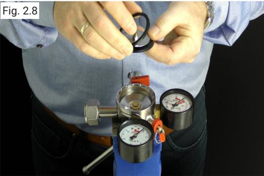
Separate the diaphragm washer from the diaphragm.
