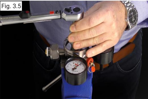
Tighten the new Cartridge with a torque of 5 Nm ( $\pm 0.5$  Nm) by using the service tool and a torque wrench.
