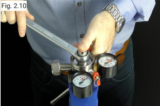
Turn the service tool counterclockwise by using a 24 mm spanner.
