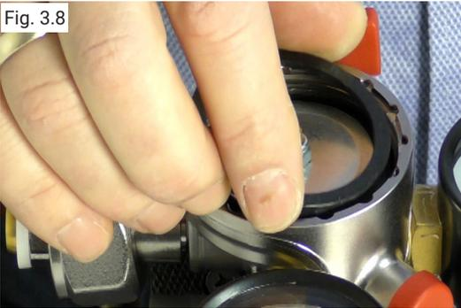
Place the reused Washer for Diaphragm on top of the Diaphragm – with the groove facing down like illustrated on the picture.
