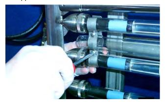
7. Disassemble the 4 hex head screws.
