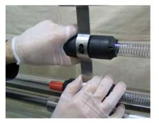
**4.** Place drip tray under Wiper System. Disconnect the tubing.
