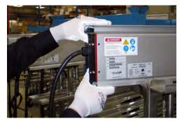
**13.** Install screws on sides of endcaps, hand tighten all 4 screws until contact is made with
