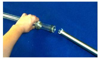
**11.** Undo 2 set screws and remove clamping piece from sensor assembly. DO NOT disassemble any further.
