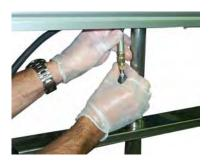
**12.** Hold the adaptor and tighten the hose swivel nut until it seats, tighten an additional ¼ turn.
