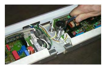
8. Lift Ballast tray up to remove Ballast.
