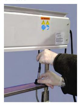
**6.** Loosen screws on sleeve bracket at the end opposite of the sensor.
