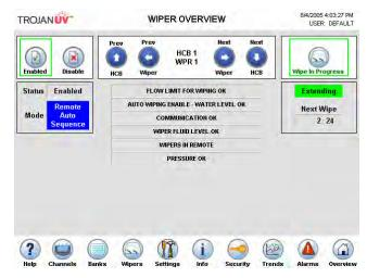
The control of wipers on the UV system is divided into Wiper Groups. The Wiper Overview screen allows access to information and control of a single Wiper Group at a time. A Wiper Group usually is associated with a single bank of UV lamps, but on smaller systems may control wiping for 2 or more banks. The information presented starting at the top left of the screen is a follows:
