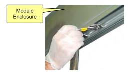
**4.** Gently pull the hoses down from the underside of the Module Enclosure along the entire
