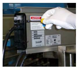
**4.** Gently pull endcaps out of Module Enclosure. If the endcaps are tight, a #2 Phillips screwdriver can be inserted into the available cross holes to act as a T-handle.
