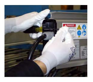
Disconnect Lamp connectors at cable end of enclosure.
