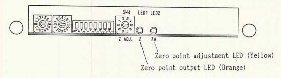
a) After turning the power of the display unit on, move the table in the direction determined in the above section to pass the zero point. Move the table very slowly (i.e. 1m/min) and ensure that the zero point signal LED comes on at the moment the head carrier passes the absolute zero point.
