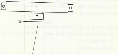
Movement direction of the head carrier (factory setting)
